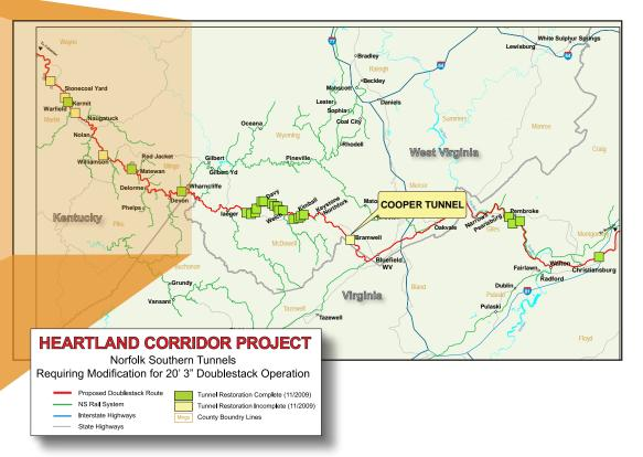
The Heartland Corridor project is raising the height of 28 tunnels, shown on the map as green or yellow boxes, to allow double-stack trains to run the route. As of late December, work on all but five of the tunnels, shown in yellow, was complete.
