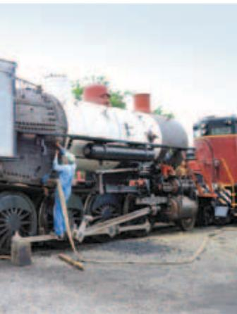
The work needed on the 4501 is not as extensive, but there’s plenty to do. One big job is to install a new firebox, including fabricating a new steel backhead. The backhead covers the back of the firebox and is what the engine controls in the cab are attached to, including the throttle and reverser gear. The restoration also will include installing new engine tubes and flues.
