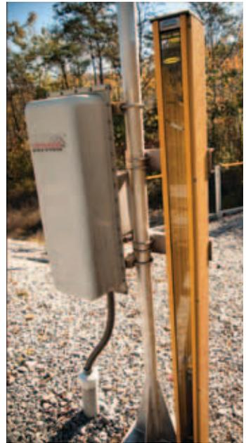
■ Data from a wheel impact load detector, aka a WILD, at the Ironto site is sent via wireless links to alert NS of a range of potential problems, from imbalanced rail cars to defective wheels. The telecommunications equipment for the WILD is maintained inside a metal hut beside the track.
