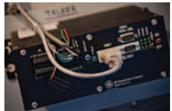
■ WILD sensors attached to the track are wired into a console inside a trackside metal hut. In photo at right, the green lights on the console correspond to individual sensors. When a train passes over the sensors, the console lights flash red to indicate they are recording data.
